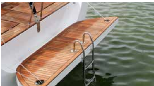
Above: The optional folding transom creates a swim platform with telescopic swim ladder
