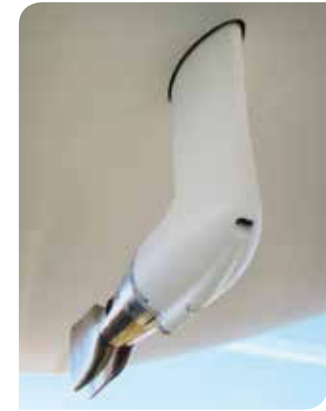
X-Yachts engine struts are faired into the hull for reduced drag and improved reliability
