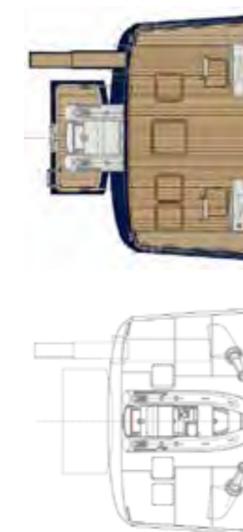
The transom folds down hydraulically to create a teak-decked swim platform, and reveal a garage for a tender of 4m.
