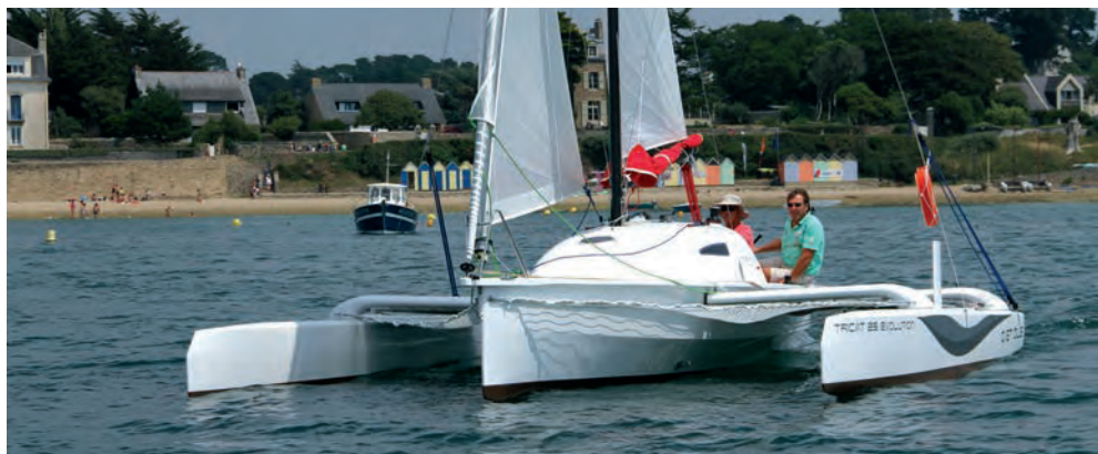
The Tricat 25 Evolution is boosted by more voluminous floats and an increased sail area.
