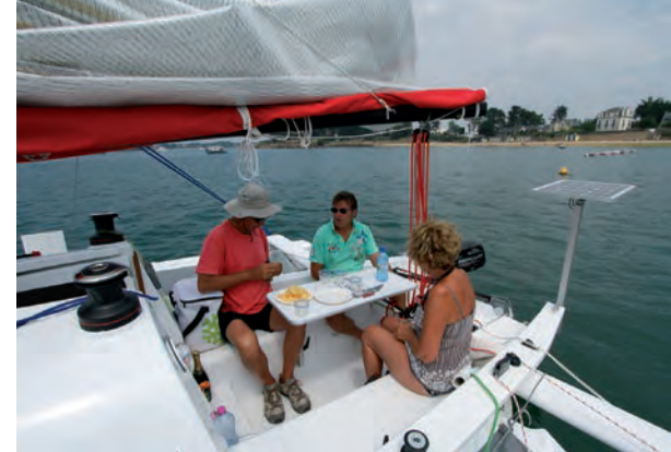
Narrow at the waterline, but a good width on deck: the cockpit is of a good size for four crew members. And then there are the trampolines for relaxing in good weather or at anchor.
