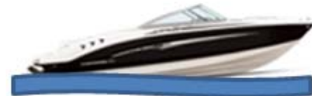
Incorrect Causes boat to "porpoise"
