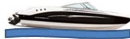
Incorrect Causes boat to "plow"
