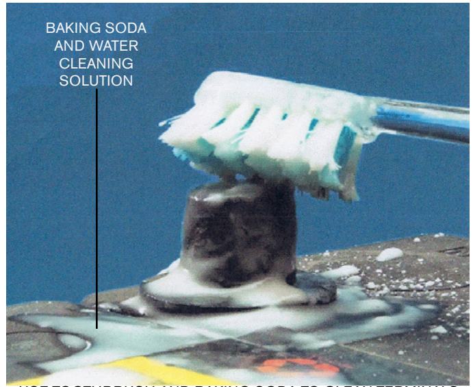
USE TOOTHBRUSH AND BAKING SODA TO CLEAN TERMINALS
