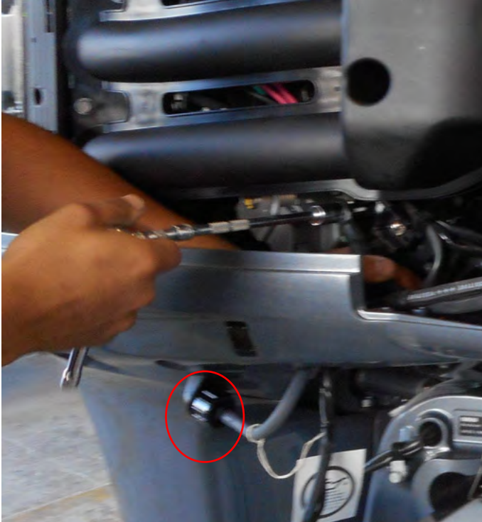
SEE FLUSHING DEVICE ABOVE CIRCLED
