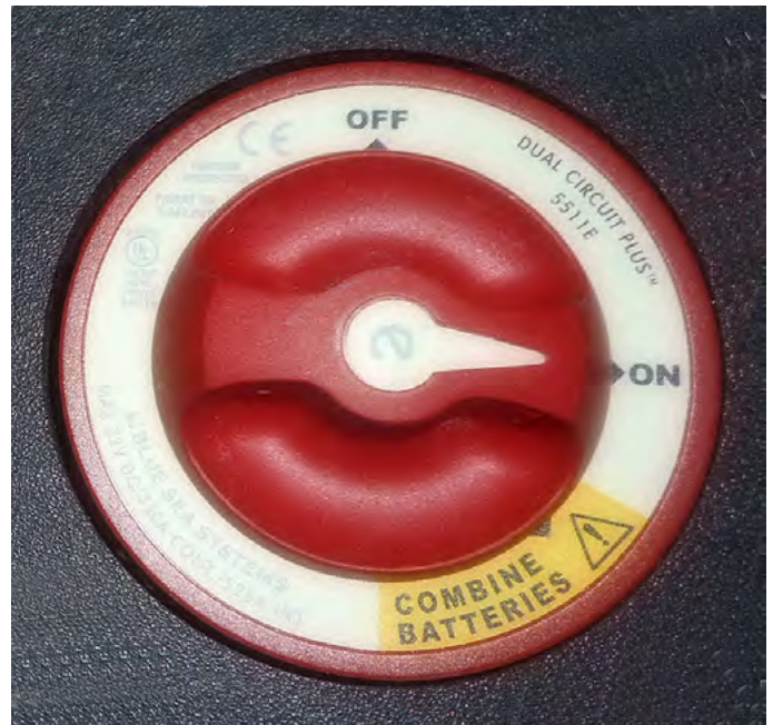
TYPICAL DUAL BATTERY SWITCH
