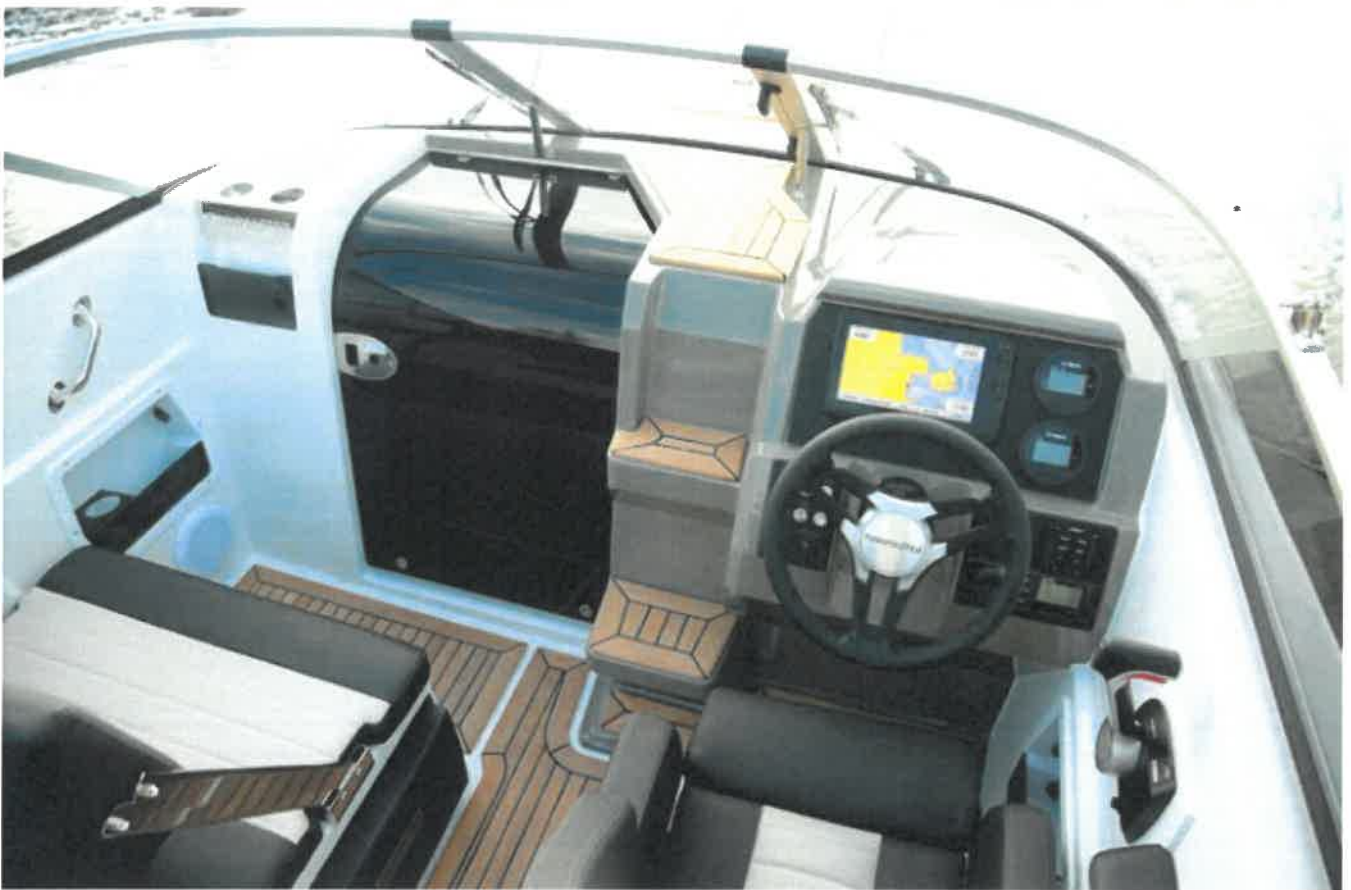
On the T6, a walk-through windscreen and moulded steps provide access to a teak-laid foredeck
