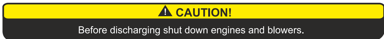
Figure 4. A warning plate about shutting down engine and blowers before discharging the fixed extinguishing system.
