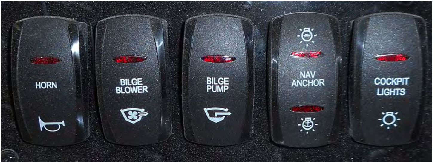
PORT SWITCH PANEL
