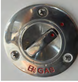
COMBO FUEL FILL/ INTERNAL VENT
