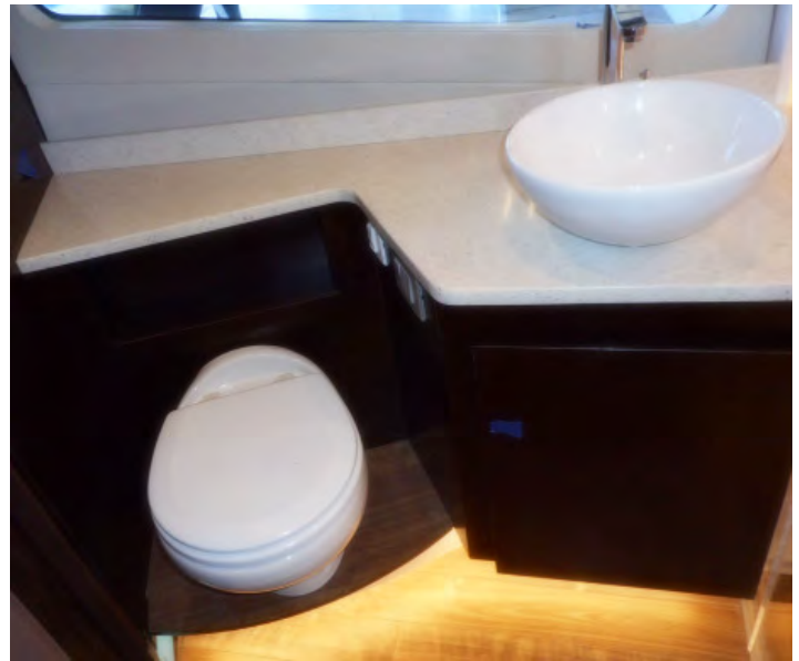
Typical Head w/ Vacuum Toilet & Vessel Sink
