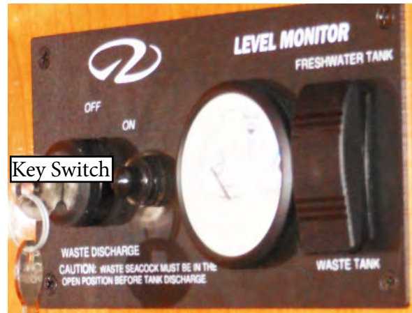
FRESH WATER & WASTE MONITOR WITH OVERBOARD DISCHARGE
