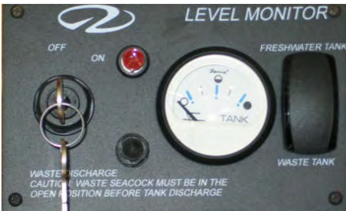
TYPICAL WATER/WASTE MONITOR PANEL
