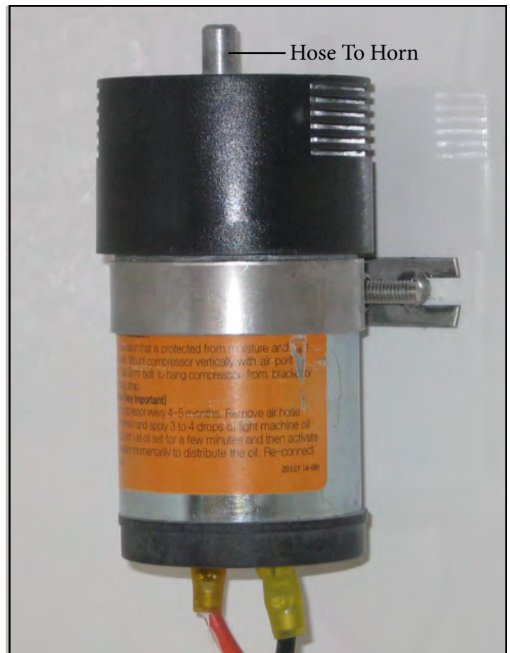
Typical Air Horn Pump
