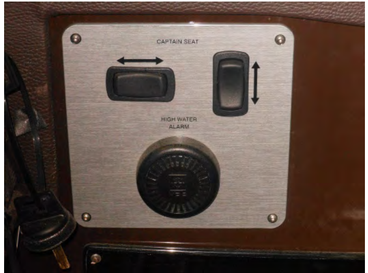
TYPICAL CAPTAIN SEAT SWITCHES
