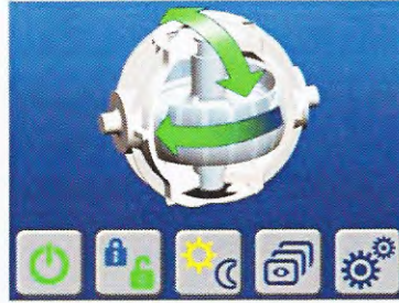
Home Screen with Arrows for flywheel spinning and stabilizing
