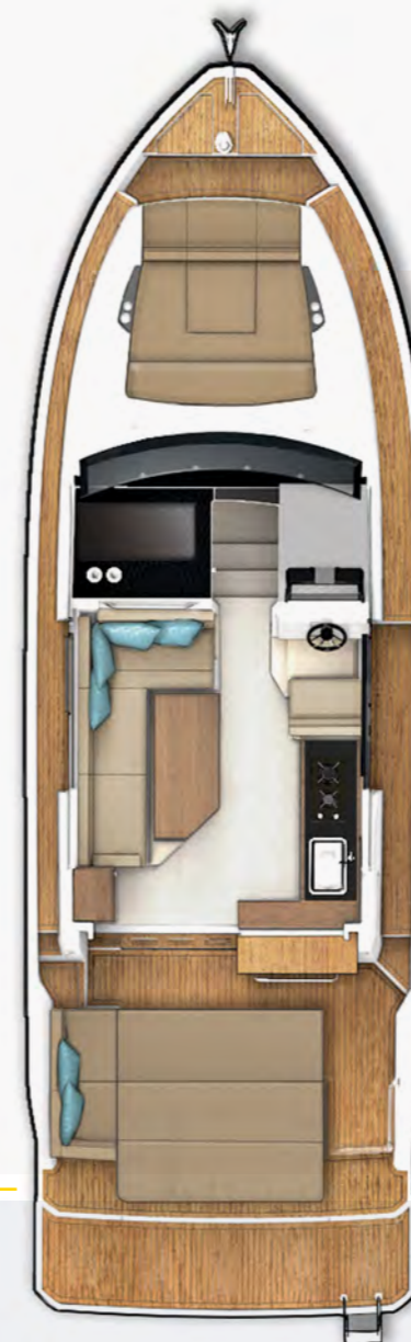
MAIN DECK option with cockpit table to be transformed into sunpad and extended bathing platform
