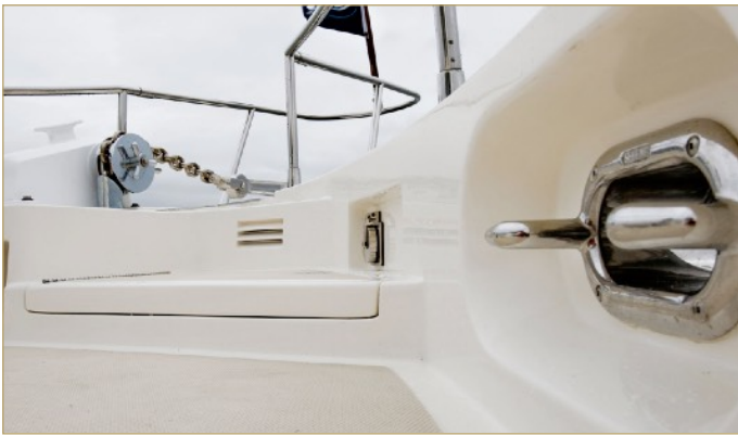
Bow pulpit, windlass, chain well & shore power
