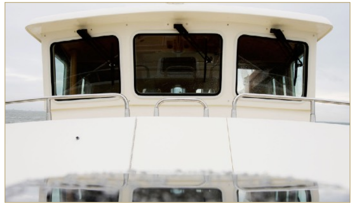
Portuguese bridge with swing door
