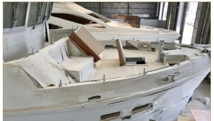
Foredeck stanchions installation
