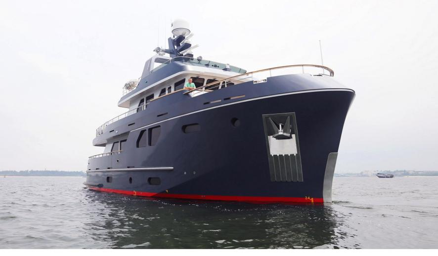
The steel-built Bering 80 motor yacht takes its design cues from proven oceangoing commercial trawlers. She features a very bold profile and her massive bow with its tremendous reserve buoyancy allows her to ride up and over large open-ocean swells.
