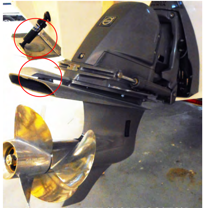
TYPICAL STERN DRIVE ANODE LOCATION
