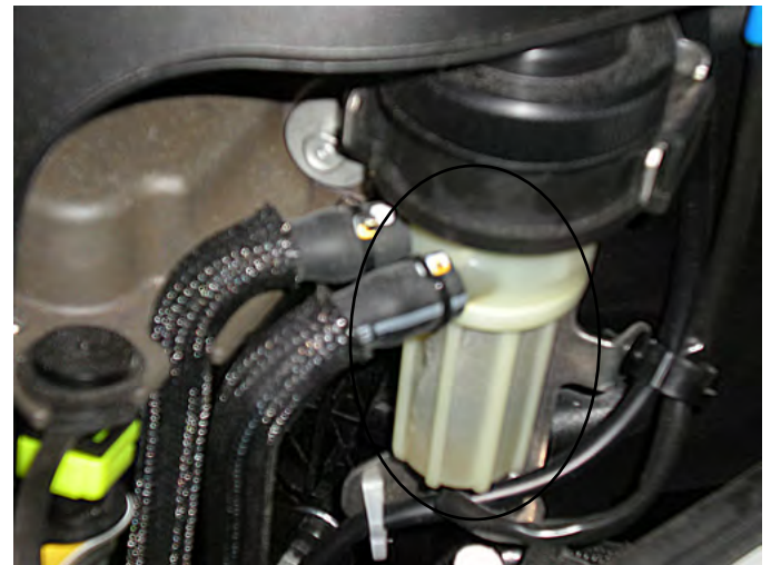
FUEL FILTER ELEMENT INSIDE FILTER BODY
