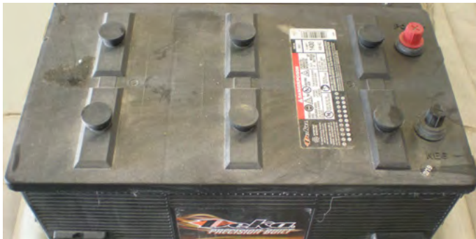
TYPICAL GROUP 8 D HOUSE BATTERY
