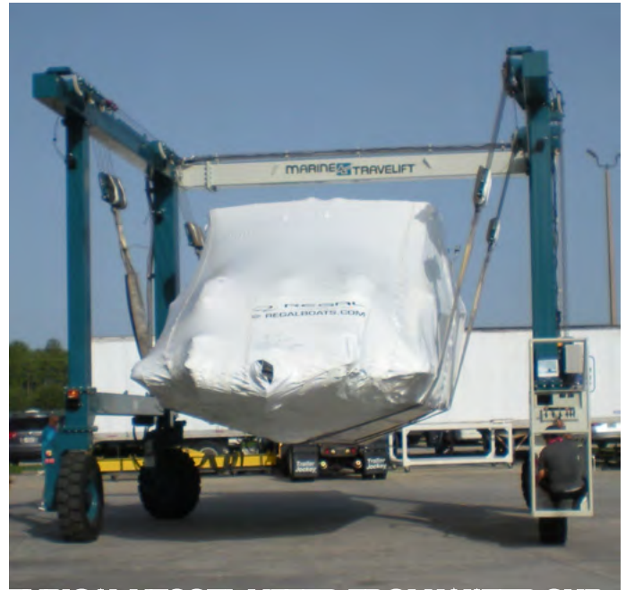
TYPICAL VESSEL LIFTED FROM WATER SUPPORTED BY LIFTING STRAPS
