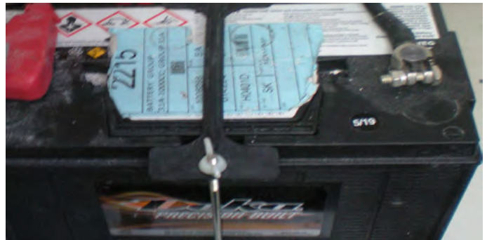
TYPICAL GROUP 31 A ENGINE BATTERY
